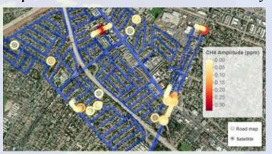
Responder<sup>™</sup> leak survey performed in a residential neighborhood, displaying leak locations, relative sizes, and user-defined ethane:methane filters. All leaks are automatically logged and prioritized by adjustable Aeris or user-defined metrics.
