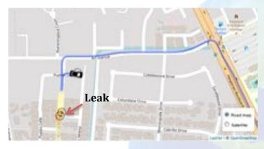
Real-time Responder™ user interface, which can be either displayed in a real-time mode or post-process mode, wherein the leak data are hidden from the driver but the route is still shown. When leaks are encountered, a marker is dropped and location logged into a list, which prioritizes leaks based on various metrics.
