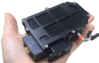
MIRA laser-based sensor engine, comprising a fixed, hermetic optical bench, integrated laser and detector subassemblies, and ultra-compact, 60cc, 13m path length optical multipass cell.
